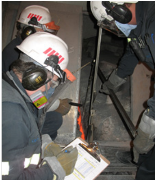
Figure 3. Ledge measurement in an AP60 cell.
